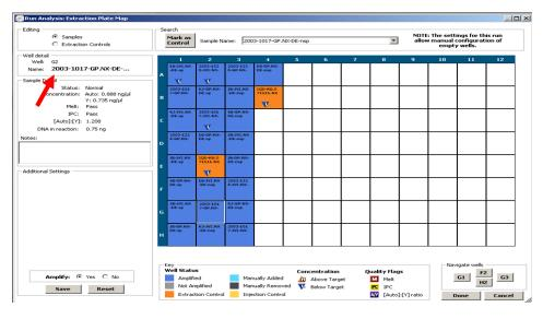
2.4.12 The next window that will pop up will concern the amplification and injection controls. Only the positive and negative controls will be utilized for this step. The positive, negative and allelic ladder (if applicable)
